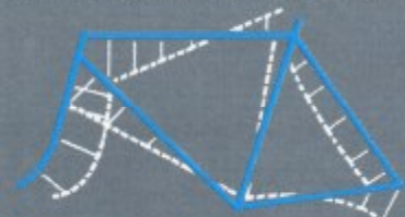
The area between the blue line (skeleton of the frame) and the dotted line illustrates the degree of stress distribution.
