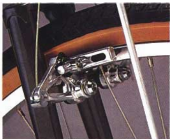
Cantilever brakes insure safe descents with heavy loads.
