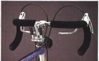
Cushioned handlebar grips, brake extension levers, and stem shifters are standard features.
