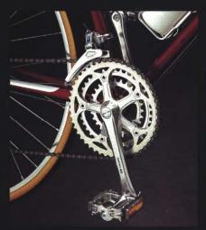
Triple alloy crank set with alloy platform pedals
