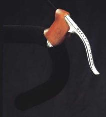
Alloy sidepull brakes with drilled levers and gum hoods
