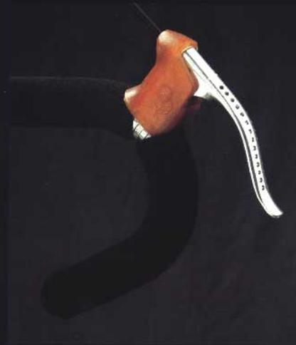
Alloy sidepull brakes with drilled levers
