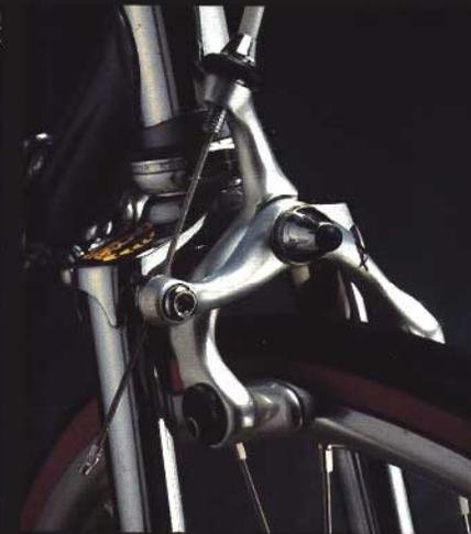
Aero alloy sidepull brakes with drilled levers and gum hoods
