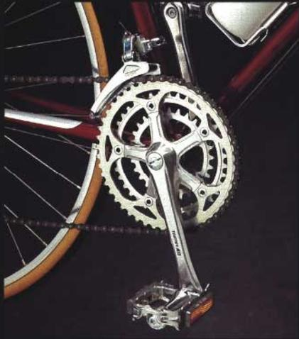
Triple alloy crank set with alloy platform pedals
