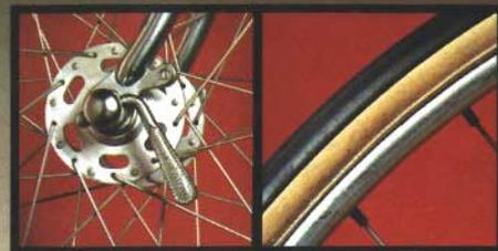
1 - Quick release wide flange alloy hubs
