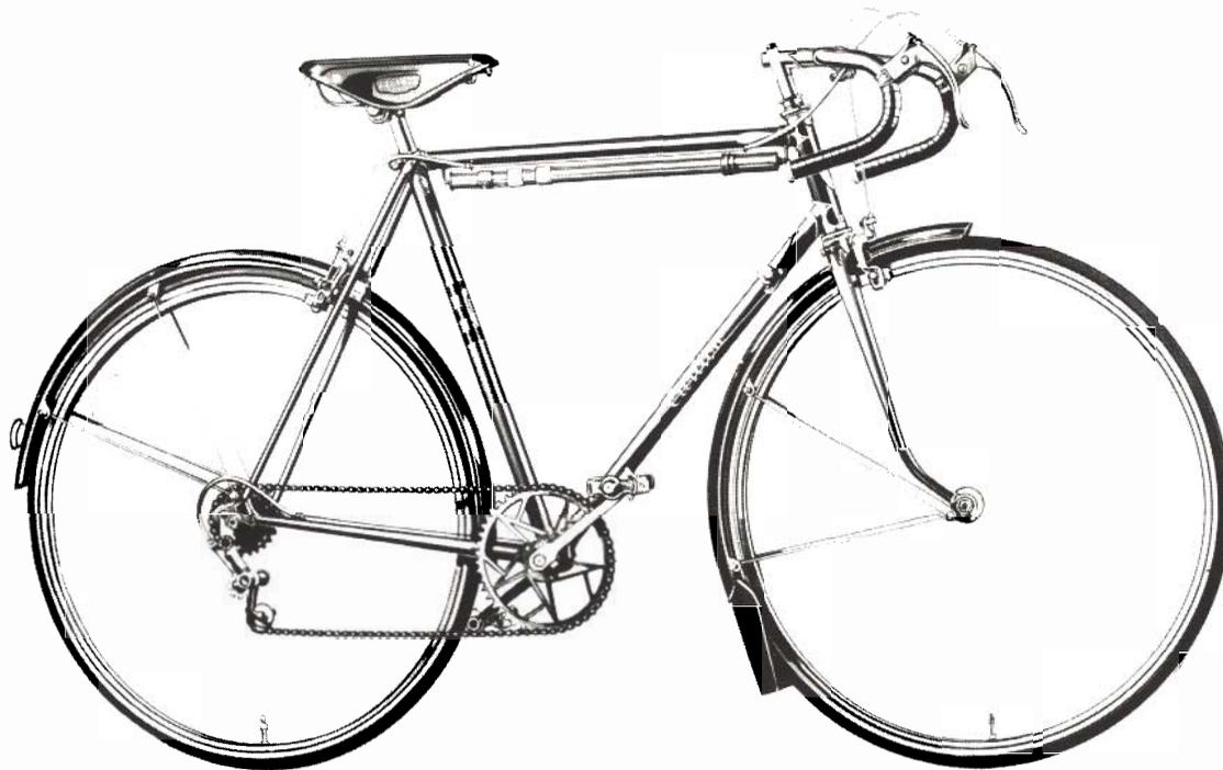
THE FRANCO-SUISSE MODEL HAS BEEN DESIGNED TO PROVIDE A REALLY LIGHT MACHINE YET AT THE SAME TIME A MACHINE DURABLE ENOUGH TO STAND THE RIGOURS OF RACING AND GENERAL CLUB RIDING. Equipped with a 5-speed gear a 23" model weighs under 24 lbs.
