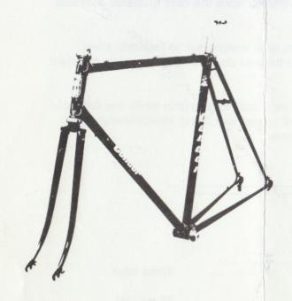
CONDOR ELITE The latest addition to the Condor Line. The Elite is a modern hand cut lug model. The beautiful lug work adds greater strength to the frame as it covers a larger brazing area.
