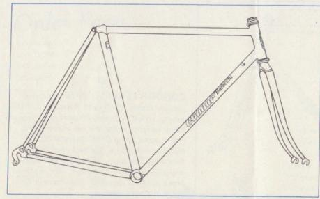
The Barracchi frame is approx. %lb. lighter than the normal lugged frame. It has proved to be very popular for use in short distance road and pursuit events. This frame is made to your personal specification and colour finish.
