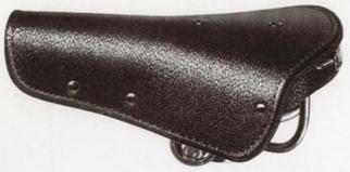
Mattress spring construction on two-wire frame with tailored felt and  $\frac{1}{4}$ " thick non-aborbent rubber interlay, the top covered with finest quality leathercloth.
