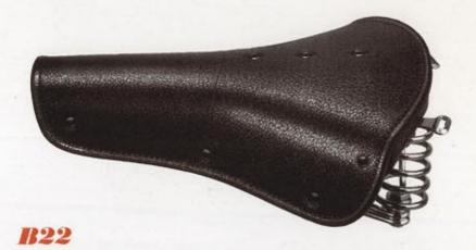
Multi-mattress spring construction in full girder frame mounted on four-wire bracket with two rear coils. Tailored felt and  $\frac{1}{4}$ " non-absorbent rubber interlay, the top being covered with finest quality leathercloth.
