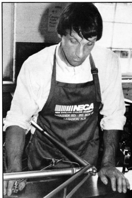
Figure 2: First base (at seat cluster): scribe tool was adjusted for light grazing contact at Home Plate (bottom bracket); seat tube is then bent (using bending bar, a.k.a. "Big Bertha," in photo at right) to bring First Base to the same level.
