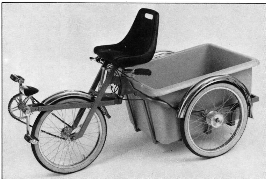
Figure 5: On this semi-recumbent HPUV, the single front wheel serves as both driving-wheel and steering-wheel. To accomplish this, the frame is articulated via an ingenious hinge/linkage under the seat. Components include a 3-speed front hub, disk brakes on the rear wheels, and a removable cargo container. Overall length: 59 inches; overall width: 31 inches. The design has passed through several prototype stages and is under consideration for commercial manufacture. Designed by Ivo Lucic, Krankenhausstr. 36, 7910 Neu-Ulm, West Germany.
