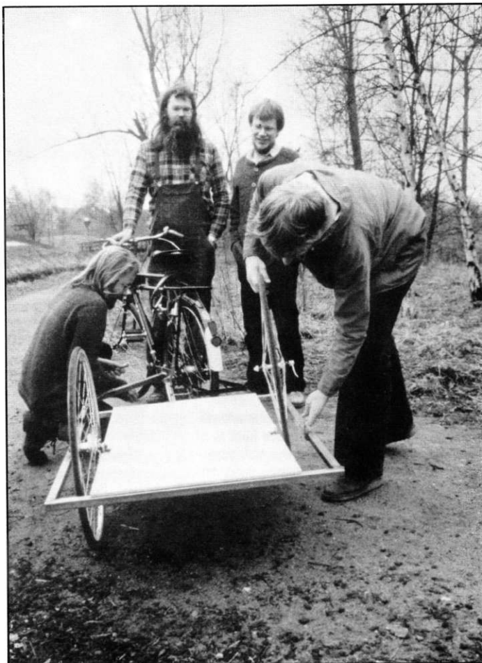
Figure 8: A trailer designed by a German university group especially for owner-builders and for easy storage when not in use. When the two quick-release wheels are removed, the basic frame—including the side-hitch attachment to the bicycle—lies all in one plane, making a very compact, flat package. The frame is welded aluminum, but a riveted model was also designed. A modified automobile ball-joint trailer hitch is used for the coupling. In 1985, a television "how-to" presentation of the construction process brought in hundreds of responses. Universitat Oldenburg, c/o Falk Riess, FB8 Postfach 2503, 2900 Oldenburg, West Germany.
