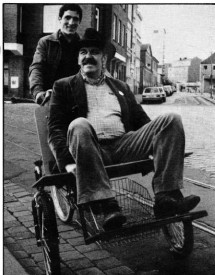
Figure 4: This model is designed primarily to transport the handicapped, and was built in a small volunteer workshop. It has a stationary (non-pivoted) load chassis (the same configuration often used for pedal-taxis in Asia), and rim brakes on the front wheels. Note the basket under the front seat. Ottenser Werkhof, Gausstrasse/Ecke Nernstweg, 2000 Hamburg 50, West Germany.
