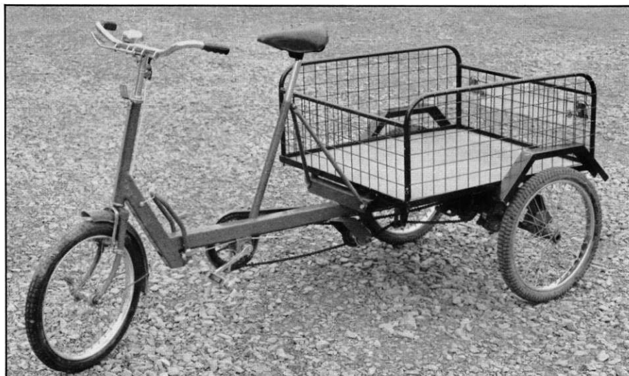
Figure 6: The OxTrike, one of the first HPUV's developed in the West specifically for Third World use. Great efforts were made to tailor the design to the materials, skills, and transport needs of these countries. The brake (note "pedal" on the main frame tube) applies pressure to both rear wheels, and also acts as a parking brake. Drivetrain includes a 3-speed transmission and differential. The OxTrike is now manufactured in about a dozen small workshops in several countries. The project was initiated by IT Transport, Ltd., The Old Power Station, Ardington, Oxon., OX12 8PH, United Kingdom. Several other groups are also actively working to develop Third World HPUV applications. 1,3,4
