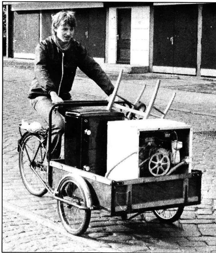
◀ Figure 2: Moving a roomful of furniture or even a washing machine is an easy task with the sort of human-powered utility vehicle (HPUV) seen here. For touring/camping, a cot and tent arrangement can be set up in the front compartment, thereby providing the world's first 3-wheeled human-powered Winnebago! Designed and built by Christian Kultz, Dammstrasse 44 Hth, 2300 Kiel, West Germany.
