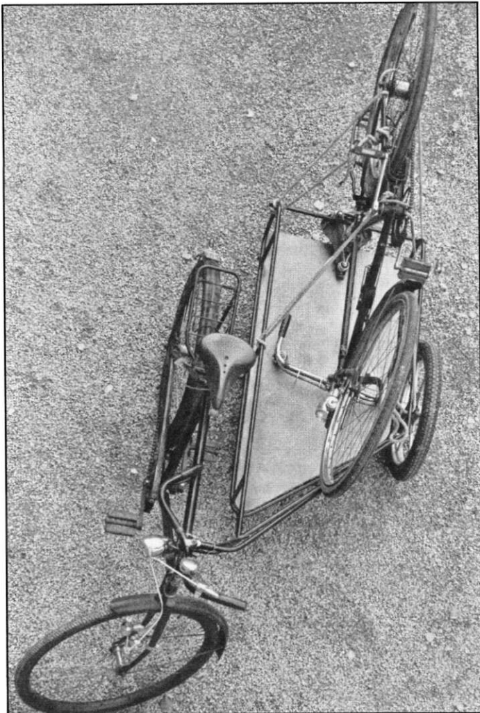
Figure 7: A detachable sidecar carrier, with two-point mounting to the bicycle. Sidecar's single wheel is a 20 inch heavy duty model. The bicycle shown here is the classic Swiss military type. Variants of this configuration, with a passenger's seat on the sidecar, are common taxis in Indonesia. Fahrradbau Stolz (small workshop), Allenmoosstr. 34, 8057 Zurich, Switzerland.
