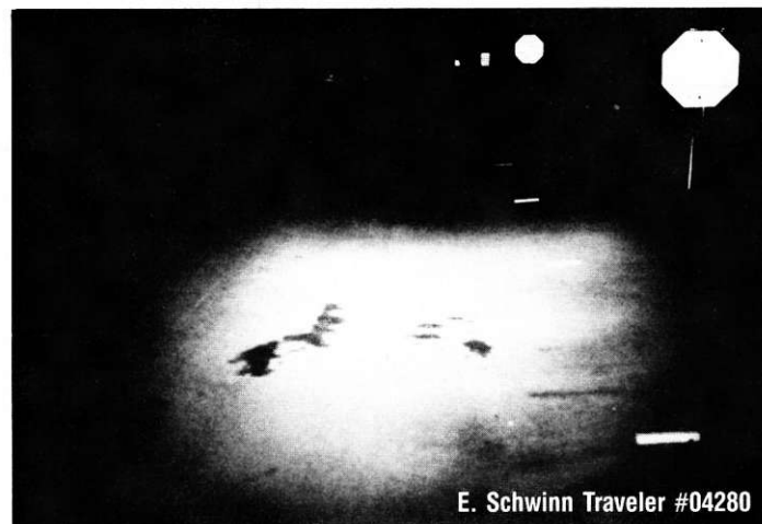
Figure 5: On-the-road beam patterns of seven lights, spanning the range from brightest to dimmest; all photos taken with same exposure settings and camera location. Drawing shows photo setup.
