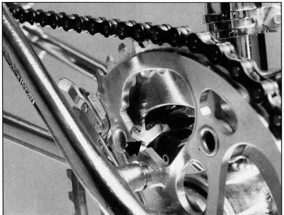
Figure 6: Chainring pawl (at arrow) shown passing through the control cams in the selector assembly.
