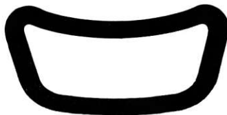
Figure 1: Fiamme Red Label Tubular rim. Cross section area = 0.1031 \text{ in}^2 .
