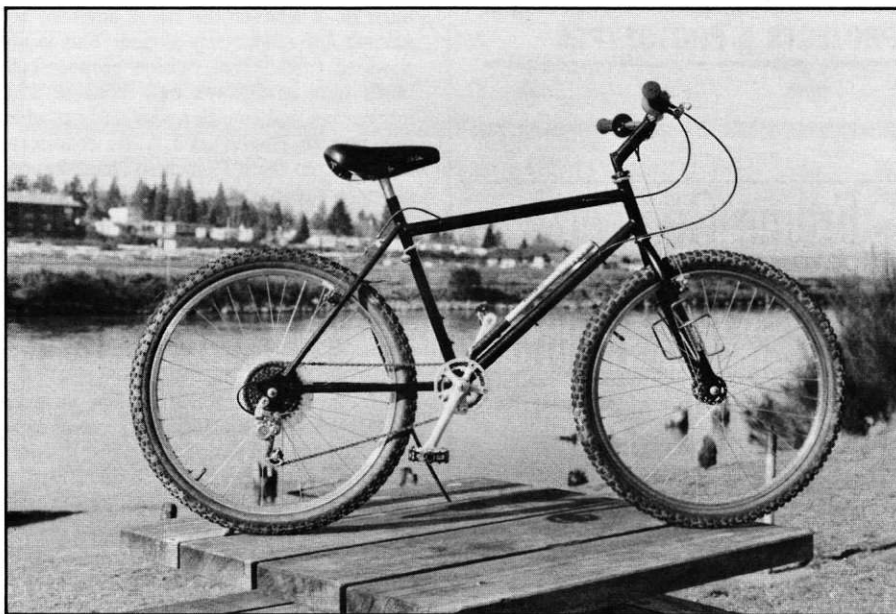
Form follows function on this rough-trail bike. Short chainstays give best traction for steep hills; high bottom bracket and minimal chainring optimize ground clearance.
