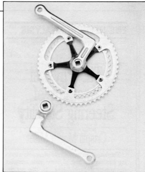
The P.M.P. crankarm has no moving parts — just a longer piece of metal "to allow greater ease on the upstroke."
